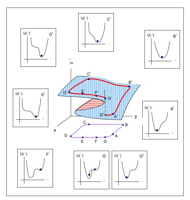
Before looking at catastrophes in general, we consider the behaviour of a mechanical system near a cusp catastrophe, one of simpler possible types. Fig 3 shows the variation of a potential energy function U( $\overline{}$ ) and its stationary states  $\overline{}_{eq}$ , for various points of a closed circuit ABCDEFGG' in control space.
